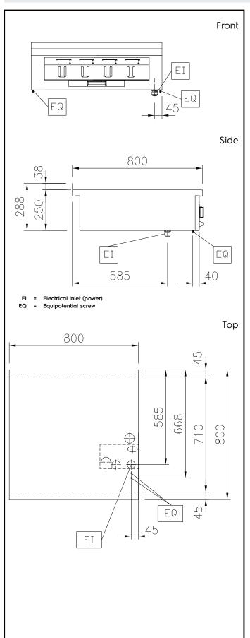
**Electric** Supply voltage: 400 V/3N ph/50/60 Hz 12 kW Electrical power max: **Key Information: Working Temperature MIN:** 100 °C **Working Temperature MAX:** 450 °C External dimensions, Width: 800 mm External dimensions, Depth: 800 mm External dimensions, Height: 250 mm Net weight: 115 kg Configuration: One-Side Operated;Top Front Plates Power: 3 - 3 kW **Back Plates Power:** 3 - 3 kW
